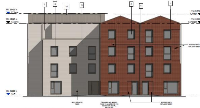
14 Block E East Elevation 1: 100
